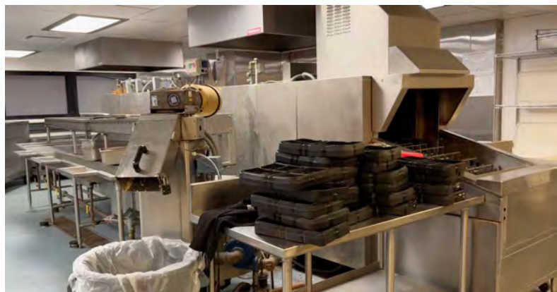
Tray wash machine minus motor
