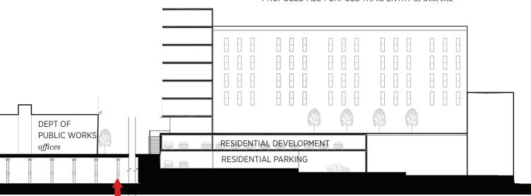
RAMP CONNECTING TO DETROIT AVENUE could serve as an entry point for pedestrians. Removal of the concrete plinth over the space of the entry would require only minor modifications.
