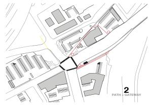
MINIMUM INTERVENTIONS would include designating the crosswalks as all-purpose trails, in addition to a ramp on the southern edge and maintaining the current entry on the north side as an entryway.
