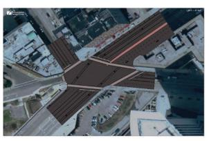
EAST END SURFACE IMPROVEMENTS include striping the intersection at Superior Ave., W. Huron Rd., & W. 9th St., plus a designated all purpose trail on the north and south sides of the bridge
