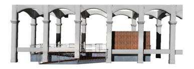
${\tt INSTALL~PLATFORMS~where~lower~crossbeams~are~not~present,} \\ avoiding~additional~structural~configuration.$
